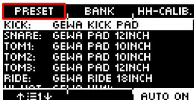
Use the dial **[5]** or the navigation keys **[8]** to select your GEWA set from the list and confirm via **[F1]**. The process is now complete and your GEWA drum set is optimally tuned to the G5 module.
